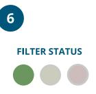
On units with filter status indicator, light should reset back to green. Reset filter monitor if necessary. See product user manual for instructions.
